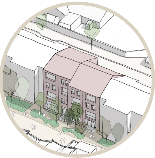
Infill buildings in underused areas of the estate, activating the street on each side by having front doors in both directions
